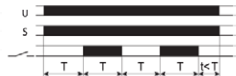
FZ31: Symmetrical recycling, OFF start, with signal contact
