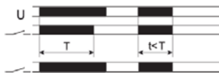
FZ20: Fixed pulse (0.5s) delayed
