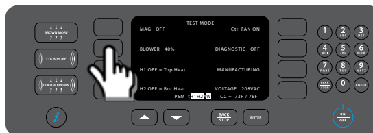
Figure 19: Test Mode: Blower Test
